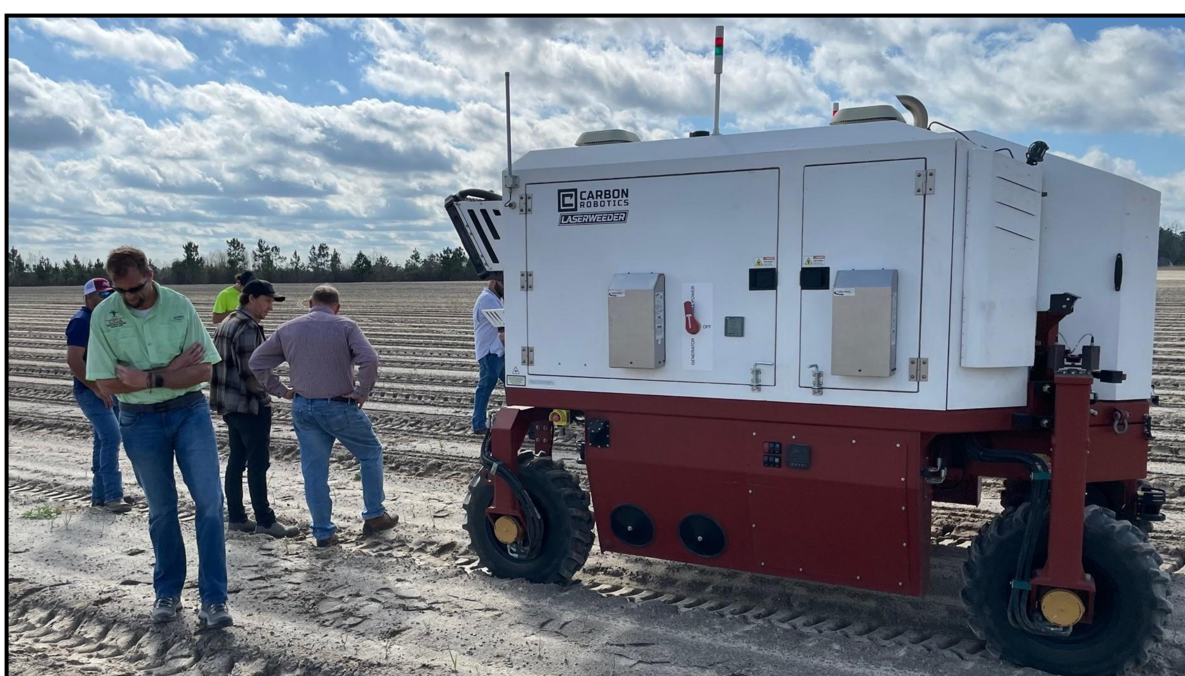
Local growers watch a field demonstration of the Carbon Robotics Laser Weeder, which uses AI technology to identify weeds and kill them with laser radiation without damaging the crop.
