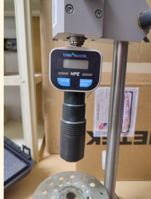
Durometer measurement (2 measurements per bulb)
