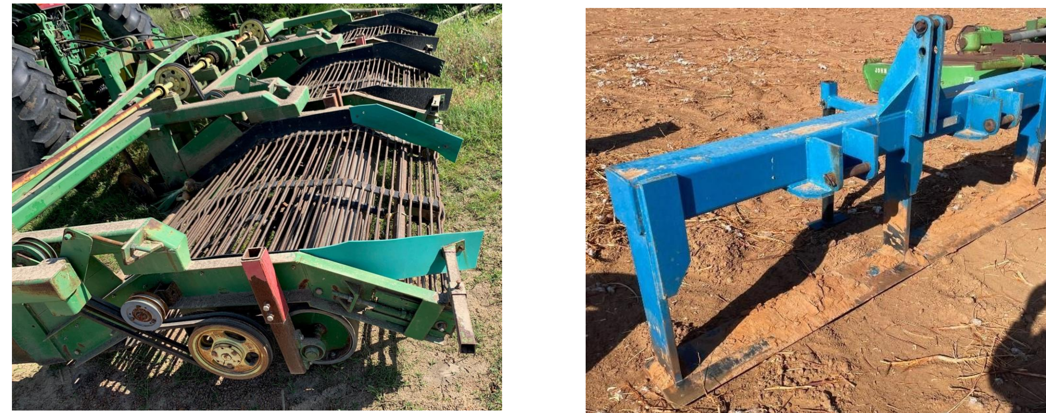
The pictures above show a typical chain digger and straight blade undercutter used in the Vidalia region.
